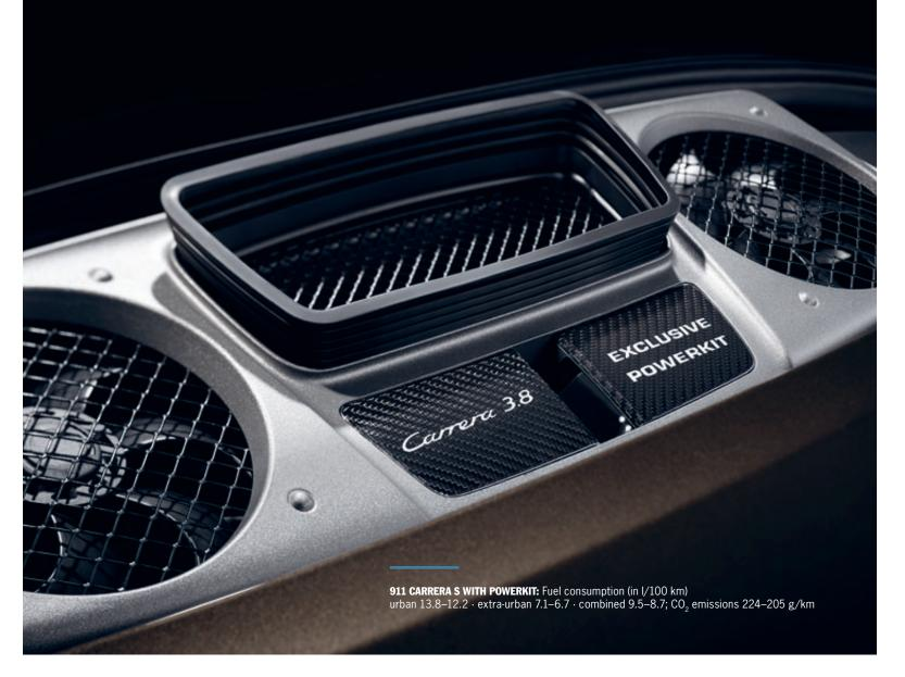
The powerkit for the engine of the 3.8-liter Carrera S of the new 911 series has been available since June of this year. Output jumps from 294 kW (400 hp) to 316 kW (430 hp), thereby reaching a level previously reserved for the cars in the GT series.
